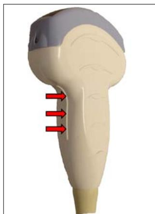
*Fig. 3: Three red arrows indicate the marker on the probe, which concurs in a standardized way with the left side of the image on the monitor.*
